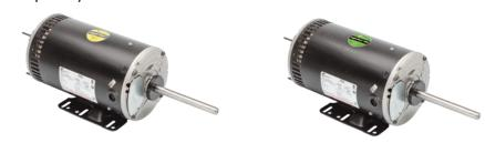
Changing voltage from 230V to 460V is easy with VCD switch. Remove two screws to open the access plate and reposition the jumper switch.
